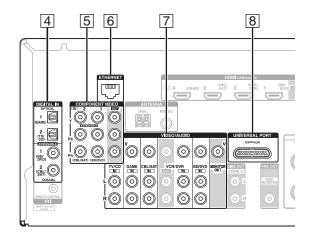
Connect your components to the appropriate jacks. The default input assignments are shown below. See "Connection Tips and Video Signal Path" for more information (>> page 77).
